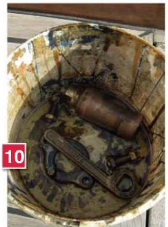
10 So that I didn't lose anything, I put the pieces into a bucket, along with some diesel which is ideal for cleaning and easing
